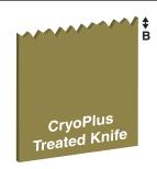
On a microscopic level, untreated tools experience aggressive wear and crack patterns. To re-sharpen these tools, a substantial area of the cutting surface (A) must be ground down to reach solid material. A CryoPlus-treated tool resists wear and cracking, and retains its cutting edge much longer than untreated tools. When sharpening a treated tool, significantly less of the edge surface must be ground away (B), resulting in substantially longer tool life.
