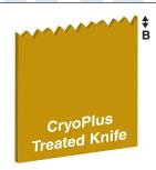
On a microscopic level, untreated tools experience aggressive wear and crack patterns. To re-sharpen these tools, a substantial area of the cutting surface (A) must be ground down to reach solid material. A CryoPlus-treated tool resists wear and cracking, and retains its cutting edge much longer than untreated tools. When sharpening a treated tool, significantly less of the edge surface must be ground away (B), resulting in substantially longer tool life.
