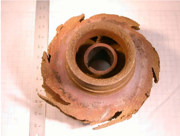
Figure 6: Severe cavitation of silicate bronze alloy impeller.
